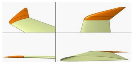
Figure 8: Raked Wing Tip with Three Panels.
