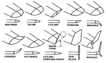
Figure 4: Different Types of Tip Devices.
